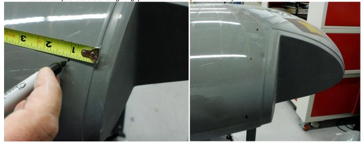
3) Using an 12" section of Fine-Line tape, use the marks to located the tape-line, ensuring that your tape-line is parallel with the existing wingtip cutouts--apply tape to the top and bottom surfaces of both marked lines.
