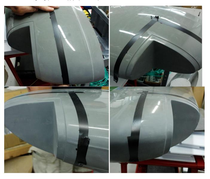
4) Once all pieces of tape are in-place and located, use a Sharpe pen to trace the inside of the tape-line (around the entire perimeter) while using the edge of the tape as a guide. Then remove the tape sections to reveal the ink-line that will be used as a guide for the cut-line.
