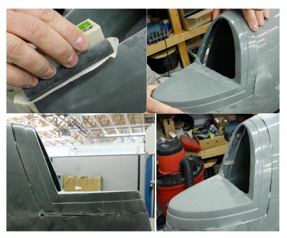
2) Using 80 grit sandpaper, sand the inside perimeter of the wingtip and the flange of the new Insert.
