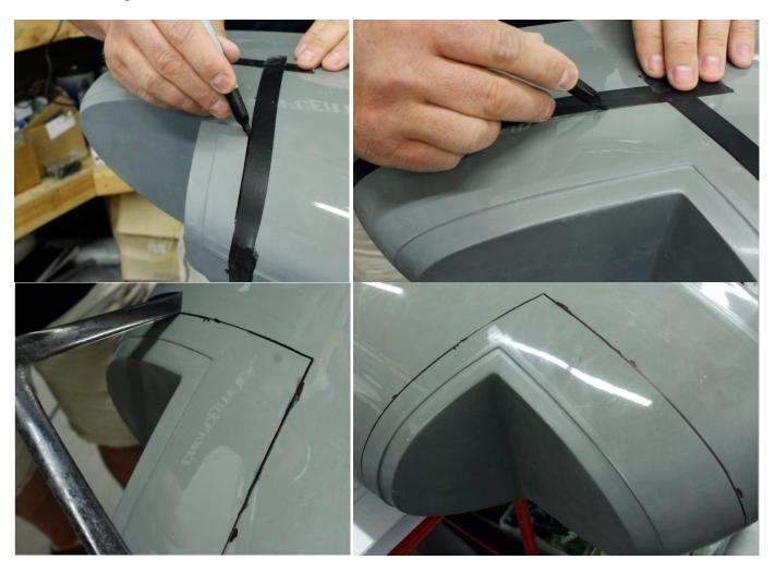
5) Using a Dremel and cutoff wheel-- cut the existing piece out of the wingtip by following the <u>outside</u> of the marked line.
