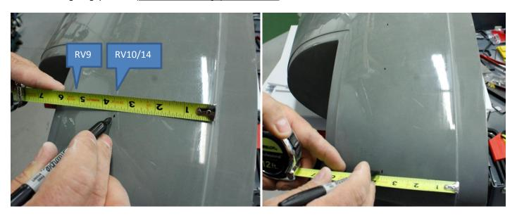
2) Using the angled-section of the wingtip cutout offset jog as the reference point, measure aft 1.0" and mark several locations adjacent to the existing wingtip cutout and mark point on the top and bottom surface.
